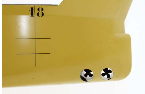
Bow tunnel thrusters on a DP shuttle tanker
